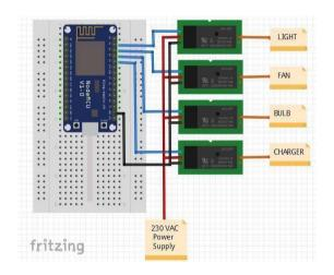
Initially we dump the required code(program) into the microcontroller using the USB port. Now we need to set the phrases for turning on and turning off the device using IFTTT. Now connections are made accordingly as show in Fig. Whenever we wake the google assistant in smart speaker or smart phone and recite the phrase there are two possibilities.(assuming normally opened configuration)
