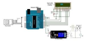
The main components of the project aside from Arduino UNO are Rotary Encoder, Relay and 16X2 LCD Display. Let me start with the Relay. Connect the IN1 Pin of the Relay Module to Pin 12 of Arduino.
