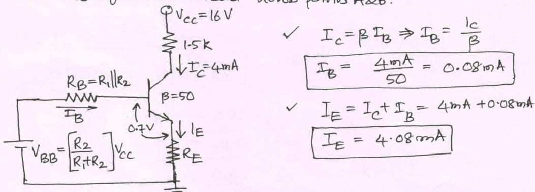
✓ KVL to o/p loop eqn :  $V_{cc} = I_c R_c + V_{ce} + I_e R_E$
