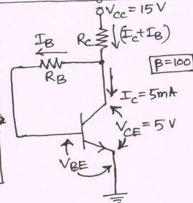
✓  $I_c = \beta I_b \Rightarrow I_b = \frac{I_c}{\beta} = \frac{5mA}{100} = 0.05mA$
