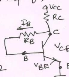
$\therefore$  The circuit with the designed values is shown here
