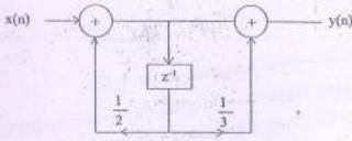
Obtain the transfer function for the above system shown in fig.
