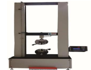
Universal testing machine (3TON load capacity, computerized operation)
