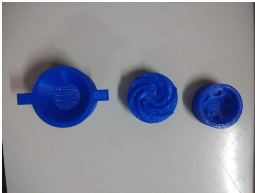
Individual parts of centrifugal pump (6 blades)
