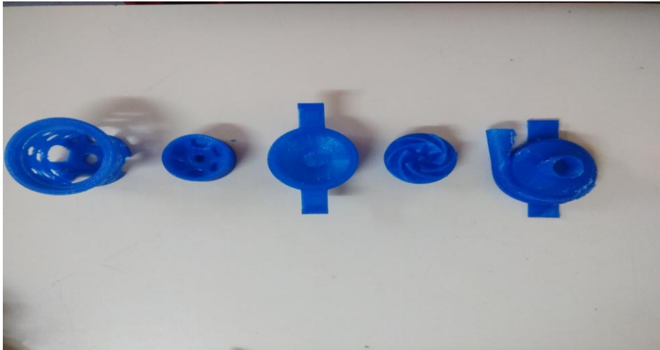
Individual parts of centrifugal pump
